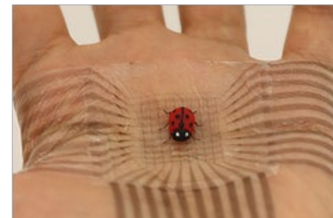
Images of stretchable electronic skin. Image credit: Amir Foudeh, Sihong Liu of Bao Group, Stanford University
